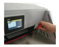
Note: when the blade is changed, the blade itself must be adjusted; if the blade is eaten too deep, it is not only easy to damage the blade, but also
