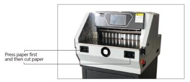
3) Start to cut after the size is entered.then pressing two CUT buttons at same time, After that, the clamper come down. When something goes wrong, stop pressing two CUT button, and press + + + the clamper and blade go back to the top. After confirming the paper is right, press two cut buttons to finish cutting.
