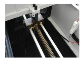
Check the stepper motor, remove the front cover, synchronize the pulley and whether the synchronization is fixed properly; adjust the limit plate on the nut, which can be adjusted back and forth until the display size matches the ruler, and then lock the fixing screw.
