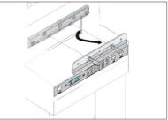
Take out a new blade, pay attention to safety, the blade is facing outward, before installing the blade, please loosen the blade at the upper end of the knife holder on the knife holder, tighten and fix it with screws in turn, and then adjust according to the cutter depth adjustment method.
